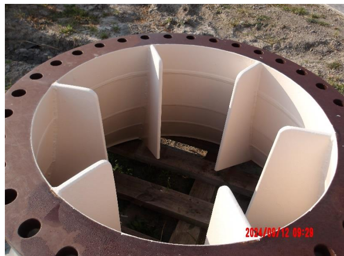
Pump #6 suction pipe with 6 vanes based on hydromodel
