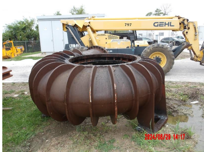
Pump #6 casing stage outside
