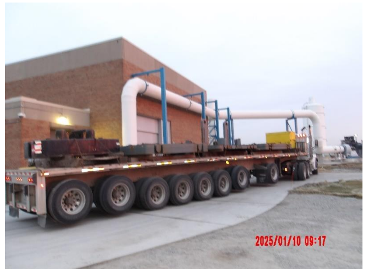
Delivery of 31.25 ton test load for overhead crane
