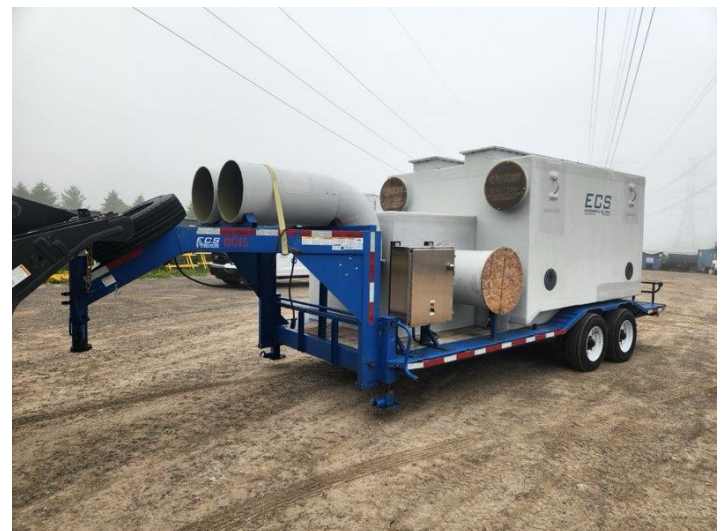
Temporary Odor Control Unit
