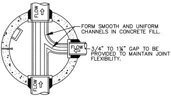
TAPS TO EXISTING MANHOLES SHALL BE MADE BY CORING AND USING A KOR-N-SEAL BOOT (OR APPROVED EQUAL).
