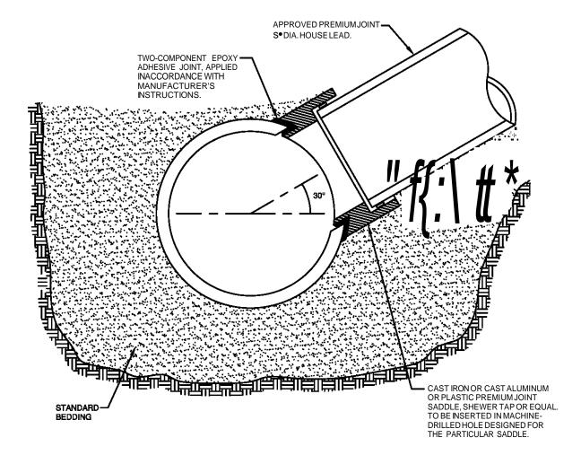
NOTE: SURFACE OF MAIN SEWER SHALL BE CLEANED WITI-1AN ABRASIVE GRINDER PRIOR TO EPOXY APPLICATION. DUE TO VARIATION OF SET-UP TIME OF EPOXY ADHESIVE WITH TEMPERATURE, ANCHOR STRAPS SHALL BE USED TO SECURE SADDLE INPOSITION IN COLD WEATHER OR WHENEVER WORK IS TO PROCEED PRIOR TO COMPLETE CURE OF EPOXY.
