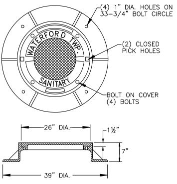
EAST JORDAN IRON WORKS HEAVY DUTY MATERIAL ASTM A48 CL.35 COVER WT., 150 LBS., CATALOG NO. 1040A PATTERN NO. 1040A, PRODUCT NO. 1040XX OAKCOSTD. 2" RAISED LETTERS, 1" RAISED LETTERS ALL RECESSED FLUSH.
