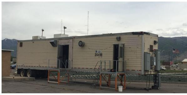
Pilot tests are needed to determine the improved digester performance (increased biogas and decreased biosolids) of CBHP with THP
