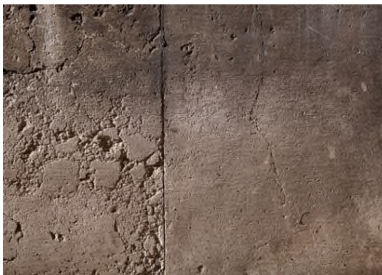
Figure 7: Side by side comparison of unaffected concrete and concrete undergoing H_2S corrosion
