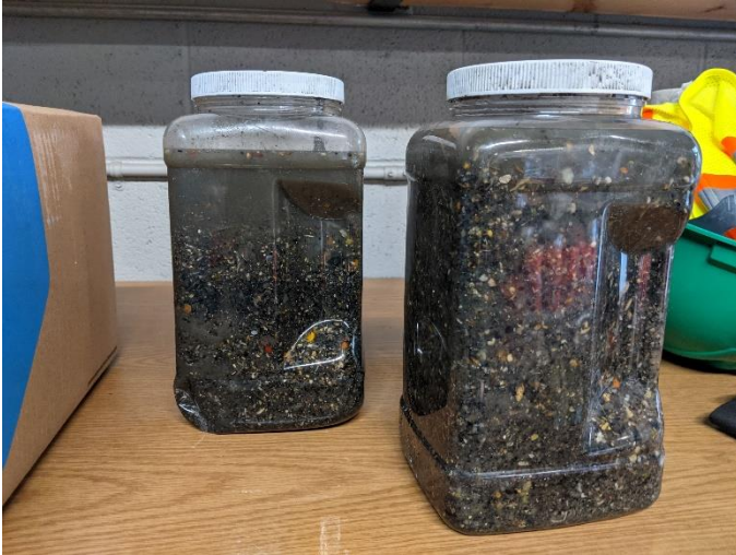
Wet Well material recently sampled appears to be asphalt roadway debris
