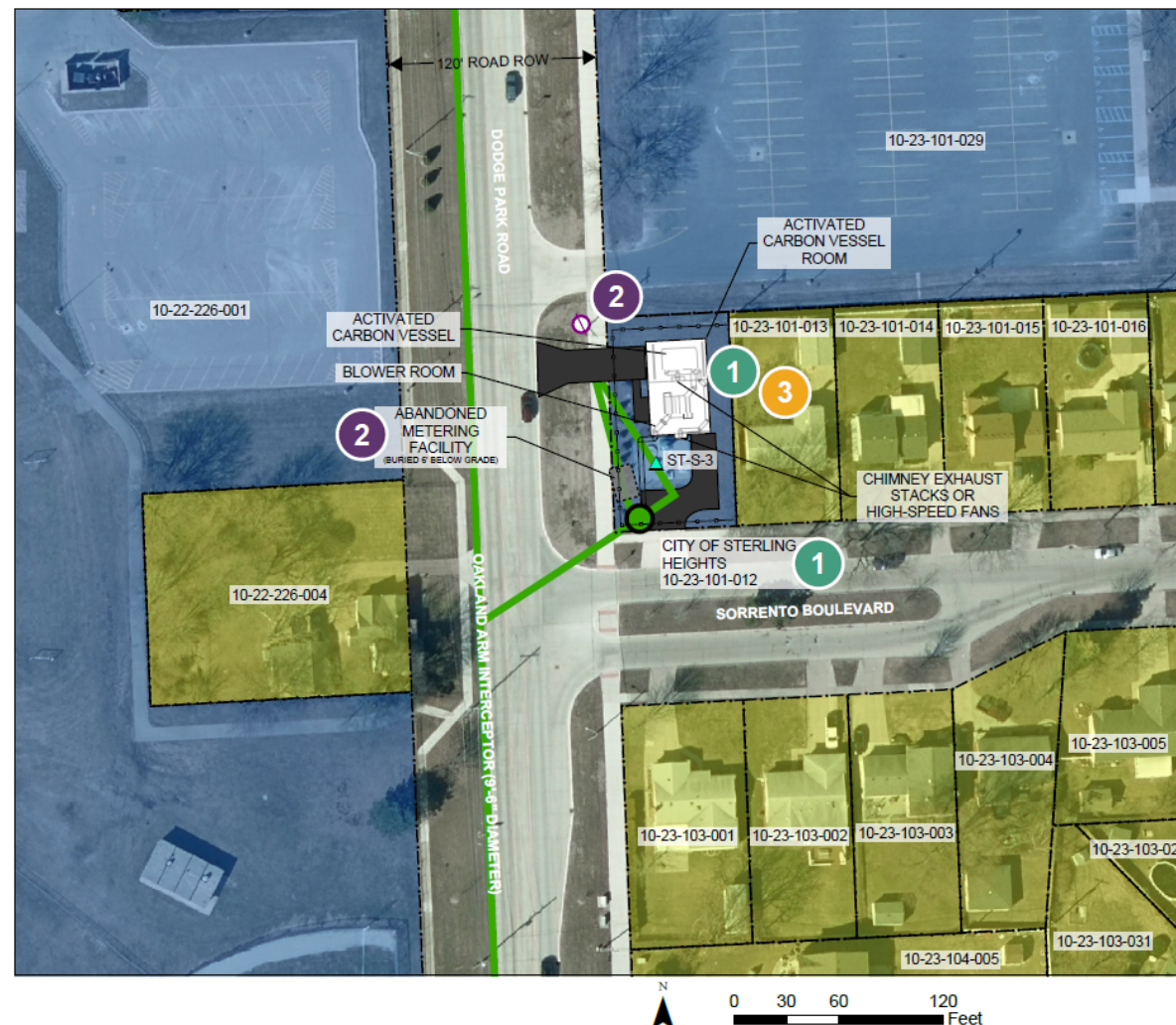
Figure ii. Activated Carbon Treatment, System Layout at Meter ST-S-3
