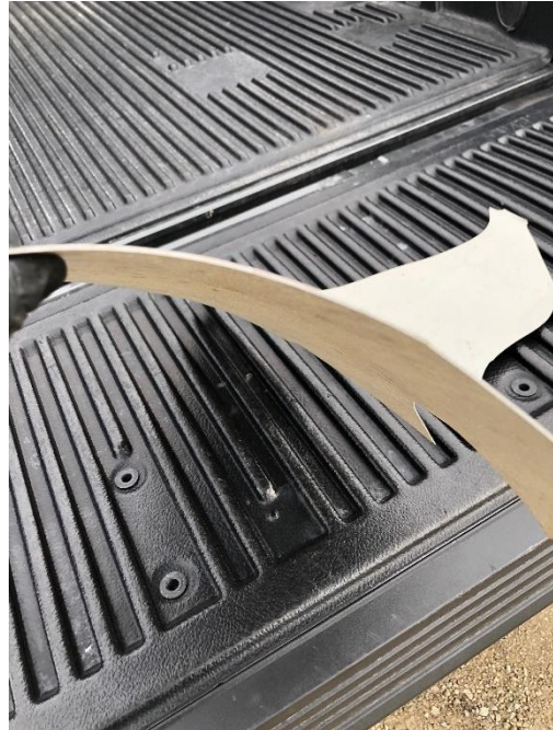
West Manifold Close-up of Pealed Coating
