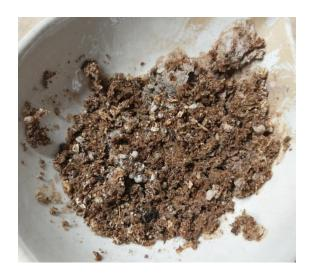
Sediment sampled from wet well during testing. Left: After oven drying to remove moisture. Right: After Loss on Ignition Testing to remove organic material.
